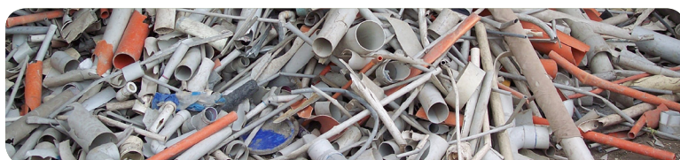
Left: Centralised post consumer pipe waiting for processing into new material. Right: PVC multi layered pipe showing recycled material at the core.
