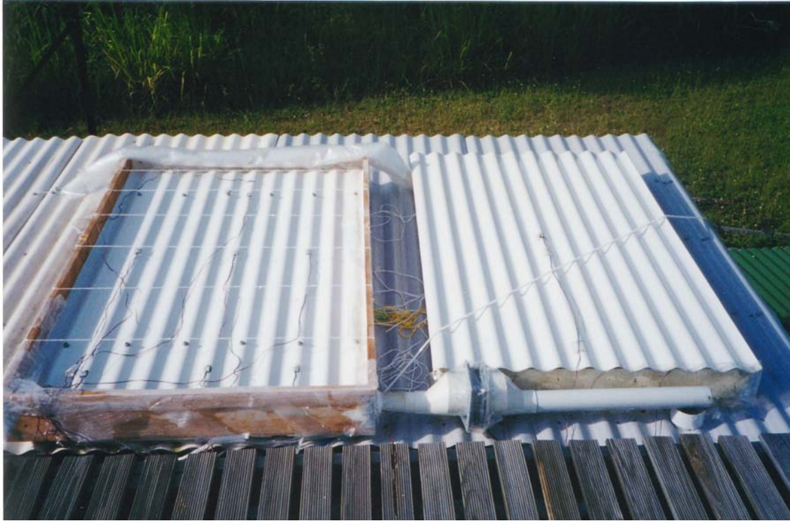
Figure 5. Wind-shielded and non-wind-shielded radiators
