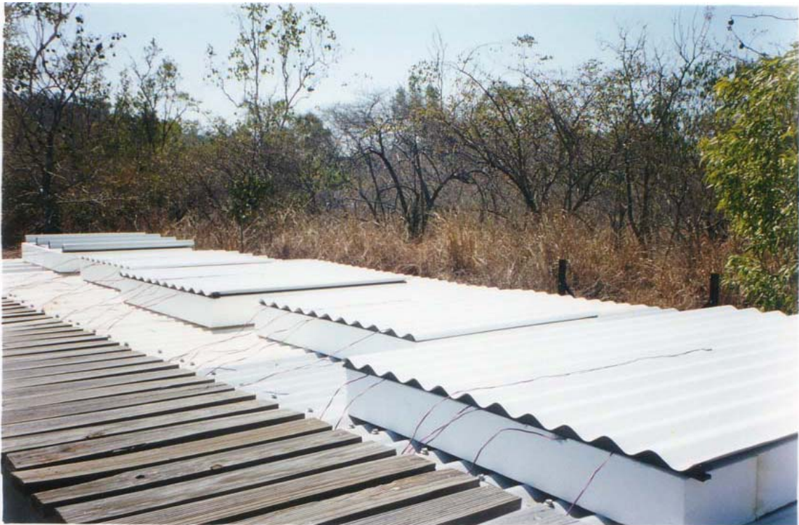
Figure 4. Non-wind-shielded Radiator under test
