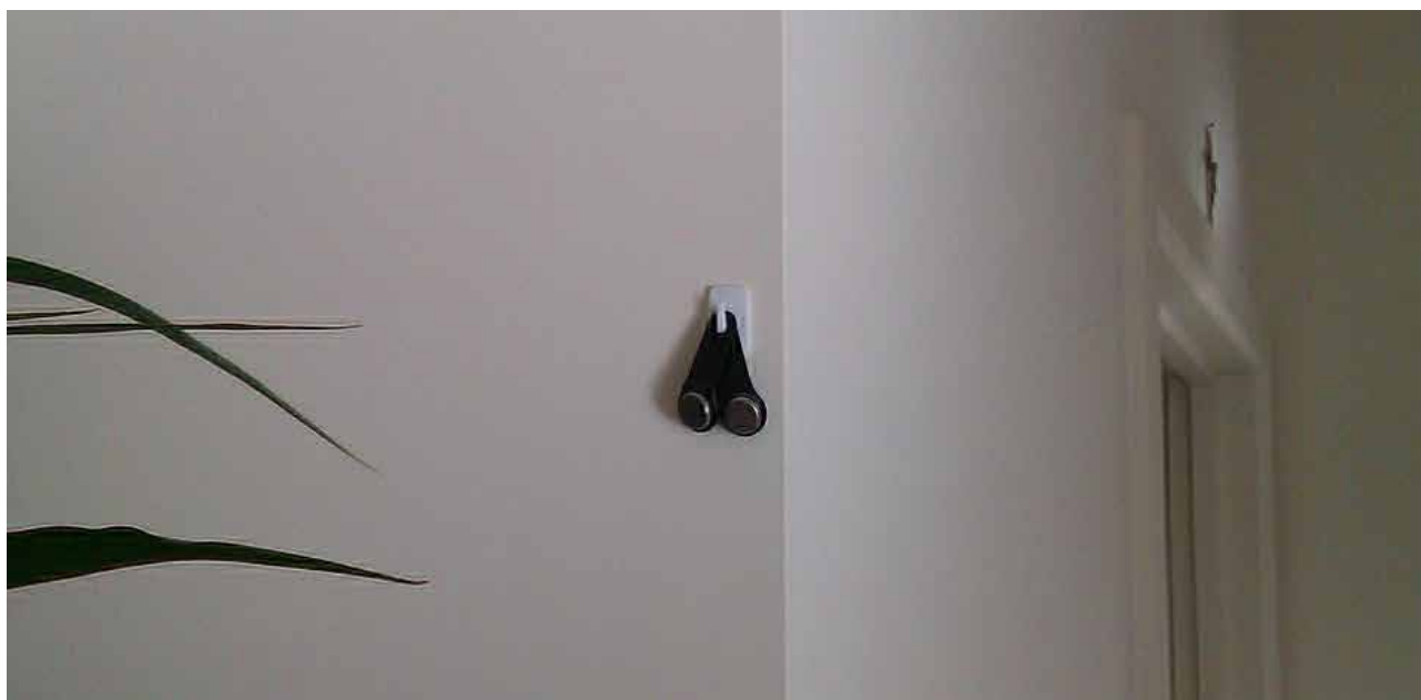
Figure 1-4 Typical ThermoChron temperature sensor installed in main living area
