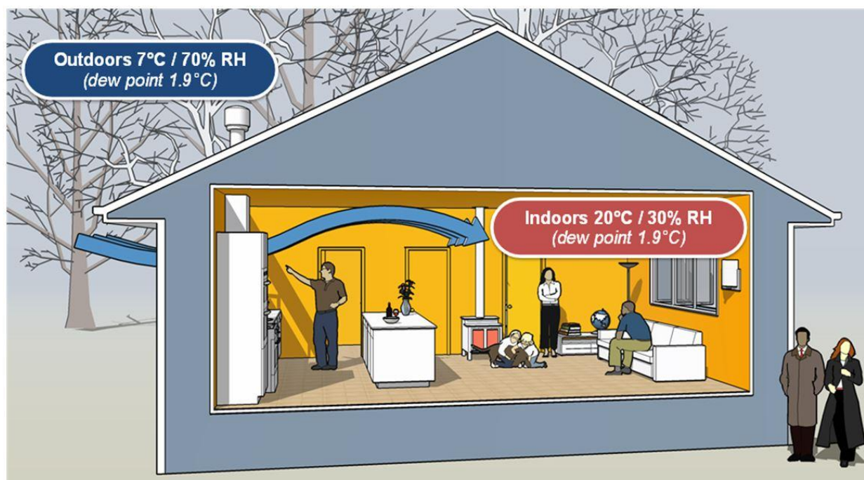
Figure 3.6 – Warmer indoor temperature lowering relative humidity of fresh air from outdoors
