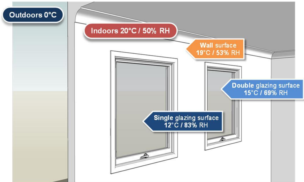
Figure 3.9 – Surface temperatures of glazing in interior heated to 20°C (outdoors 0°C)
